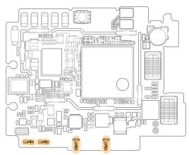
Wearable Device PCB Used for grounding between the PCB and the cover of the device
